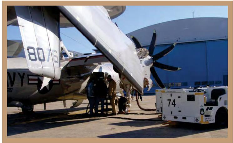
This driveable unit, with a 13 foot (4m) turn radius is ideal for operation in tight spaces and with electric drive is suitable for hangar applications. It comes with integral cable storage areas and semi-solid tires and is rated for land and shipboard use. SMEPP is air-transportable on C-130, C-17, C-5, and CH-53 aircraft.
