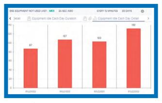
Identified \$5,303 in fuel savings per year. Four cargo loaders were tracked averaging 1.8 hour daily engine idle time per unit. Combined, that is 2,628 hours/year of wasted engine run time. That adds up to thousands per year in wasted money.
