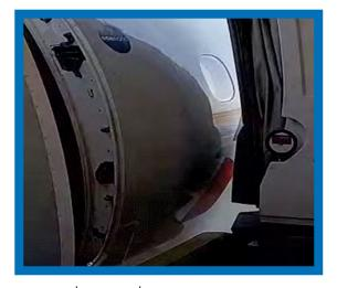
This is a \$100k to \$500k expense waiting to happen. A boarding bridge docked without the auto-level wheel deployed. iOPS from Oshkosh AeroTech can detect and notify you of these types of errors – before they become expensive problems.
